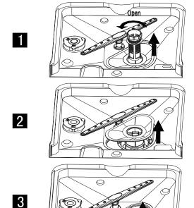
step 1: Turn the filter in anti–clockwise direction, then lift it up
