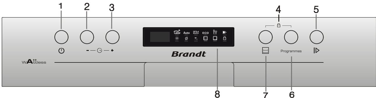
1. On/Off Button: To turn on/off the power supply.
